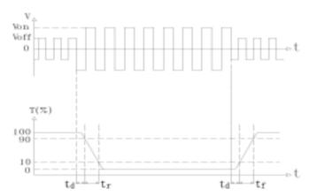
Turn on time:  $t_{on} = t_d + t_r$ Measuring Condition:
